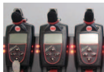
New CSAM Dosimeters receiving their 1st Charge in preparation of serving your needs
