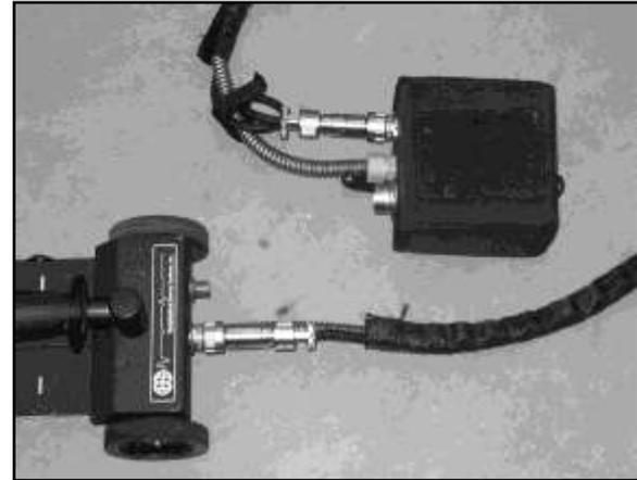
Next connect one end of the cart cable to the back of the minicart, and connect the other end to the blue padded antenna electronics box. Make sure all connections are snugged down.
